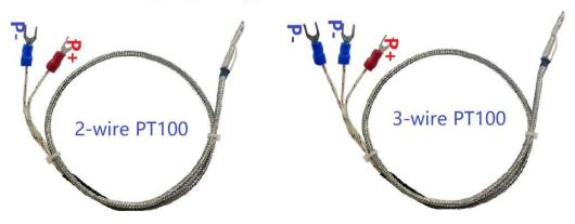
3-wire probe wiring mode: the red wire is connected to P+, and the other two wires of the same color are connected to P- and GND (the ports are not distinguished).
