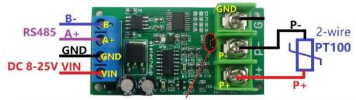
Must have a jumper cap, otherwise it cannot be measured!
