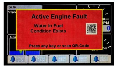
All diagnostic and emissions-related messages generated by the engine ECU, VFD, or other attached devices are displayed by the panel. The operator should be familiar with the engine manufacturer ECU and VFD messages and icons to react accordingly with respect to emissions compliance, service, and diagnostic message response.
