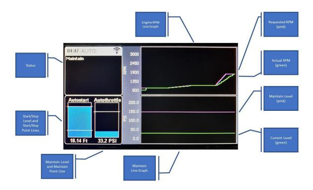
Pressing the Dashboard-2 button again will cause the display to revert to the gauge page. On a CP750-E, the gauge page can be displayed by pushing any display button and then pressing the left most button.
