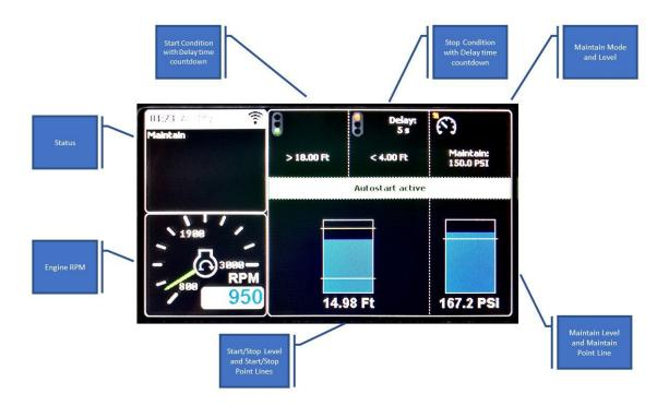
When the Dashboard-1 button is pressed again, the display will revert to the gauge page. On a CP750-E, the gauge page can be displayed by pushing any display button and then pressing the left most button.
